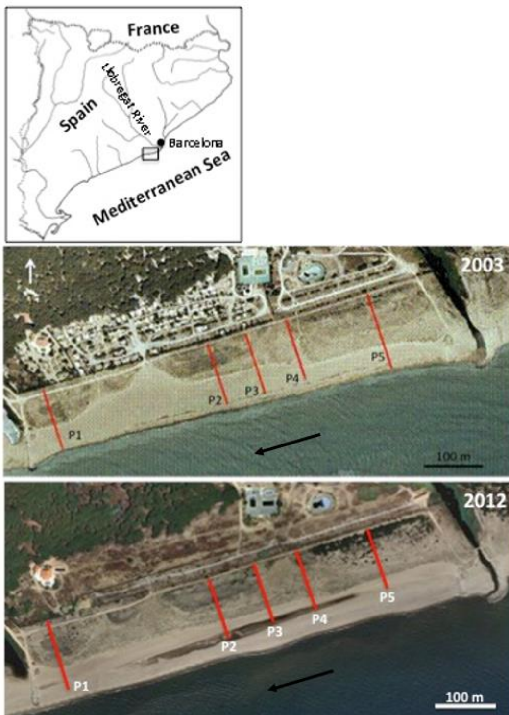
Figure 1. Location of the study area, box south of the Llobregat River and aerial view of the beach of Remolar in years 2003 and 2013 ( http://www.icc.cat/vissir3/ ). The regression of the dune system in 2003 is evidenced, mainly due to the trampling on the dunes. On this view, the red lines (P1 to P5) indicate the topographic and vegetation profiles; grain-size distribution analysis was performed in P1 and P5, and ground-penetrating radar (GPR) profiles were realized in P1 and P2. The 2013 photo shows how both the morphology of the dune zone and the vegetation in the area have increased and stabilized. The black arrow, south of the coastline, indicates the predominant direction of the coastal drift at Remolar beach, in the ENE-WSW direction.
