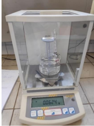
Figure 19. Picture of the KERN ABJ/ABS analytical balance with density determination supplementary set.
