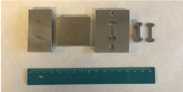
Figure 11. Picture of the dies used for molding the samples into a dog-bone shape with the application of a uniaxial pressure.
