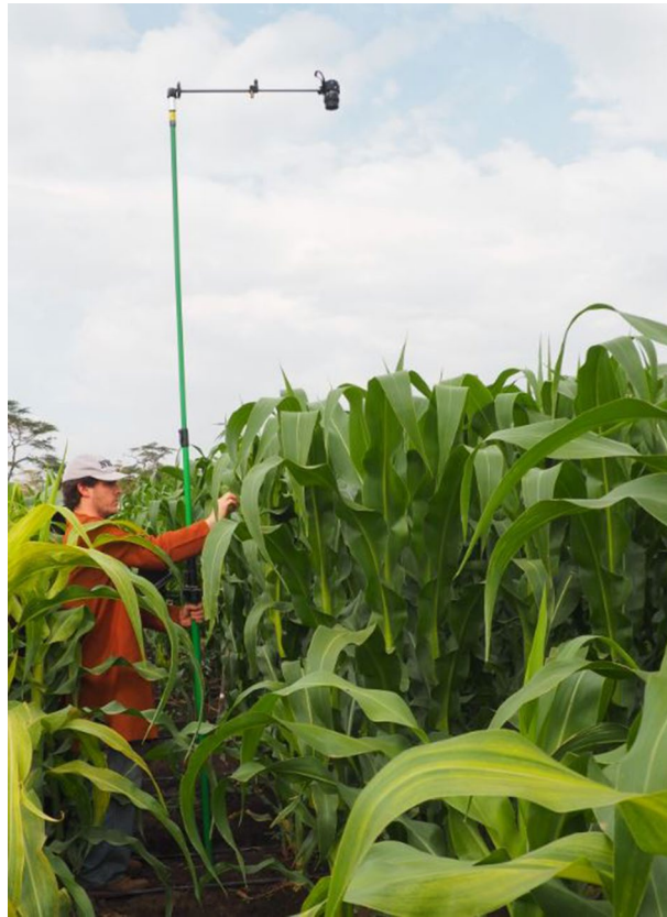
Figure 8. Ground level RGB canopy images system using the pheno-pole.
