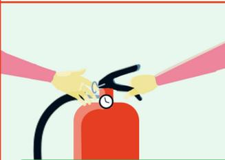
Take the extinguisher by the handle and remove the seal by pulling the ring.
