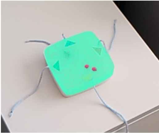
Figures 35 and 36. Hologram seen with the HoloLens superimposed to the real squared mold. On the figure on the right a delay can be appreciated.
