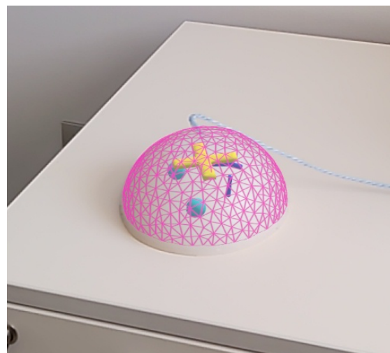
Figure 34. Hologram seen using the HoloLens superimposed to the real spherical mold.
