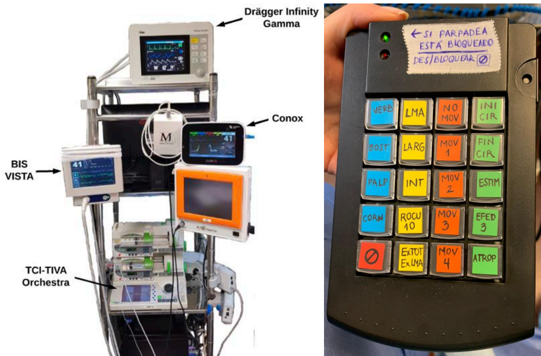
Figure 6: On the left, anesthesiology control tower, with the monitoring devices and the TCI infusion pump. On the right, the remote control used to collect data.
