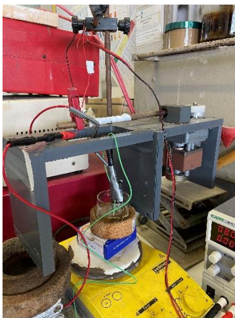
Fig 32. Electropolishing equipment used.
