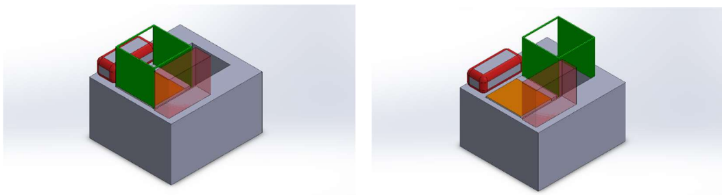
Fig. 5. Image showing the movement of the box (coloured green) from its initial position (left) at the moment the user deposits the bag and its final position (right), where the bag would fall through the hole until reaching the container.
