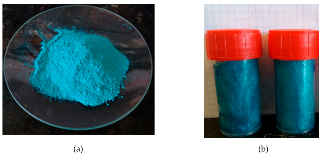
Figure 8. (a) Synthesized copper (II) oxide (CuO) nanoparticles; (b) nano-enhanced phase change materials (NEPCM) both prepared in the laboratory of the University of Barcelona.
