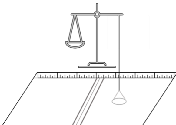
Figure 8: Pockels trough device reproduction scheme.
