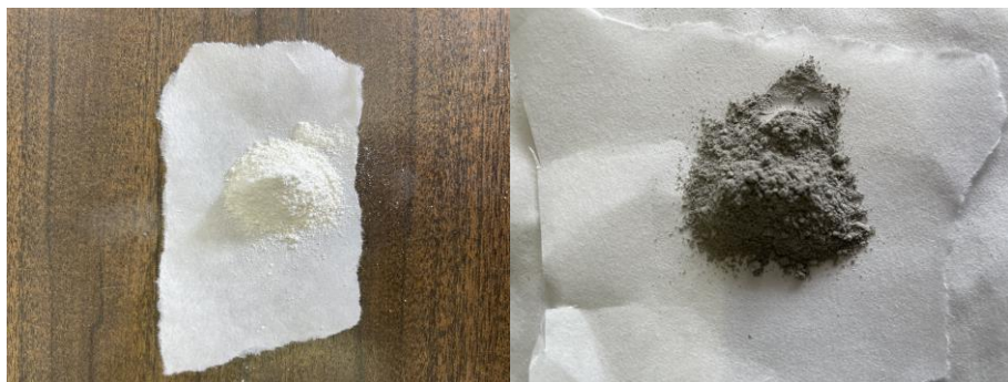
Figure 5: TiO 2 synthesized by sol-gel method after heat treatment under oxidant atmosphere (left) and after treatment under reductant atmosphere (right).
