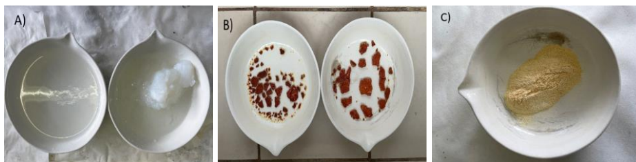
Figure 20: Dialysis process A) After neutralizing for one week (gel), B) After heating for one day at 100\text{ }^{\circ}\text{C} (apparently red \text{TiO}_2 ), and C) After grinding it in a mortar (yellow \text{TiO}_2 )
