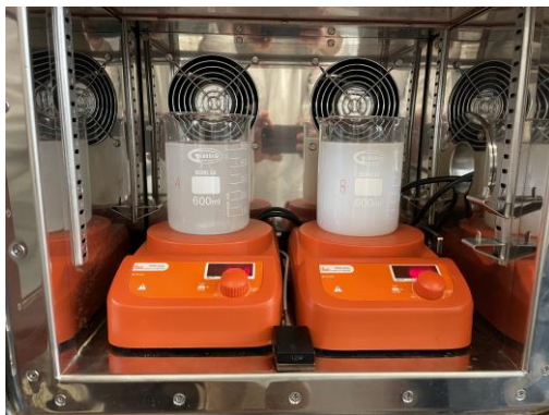
Figure 8: Experimental set-up of the photodegradation of sulfamethoxazole in aqueous suspension of \text{TiO}_2 inside a Solar Simulator.
