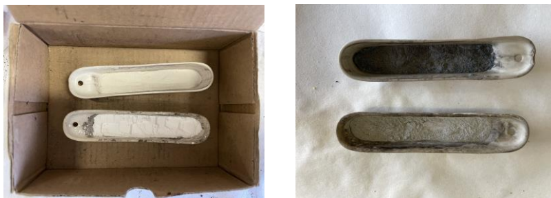
Figure 7: \text{TiO}_2 rutile (above) and anatase (below) mixed with \text{NaBH}_4 before (left) and after (right) the heat treatment under a reductant atmosphere.
