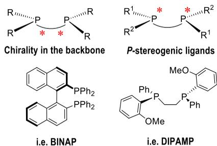
Figure 1. Diphosphines with a chiral backbone (left) and with stereogenic phosphorus atoms (right).
