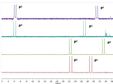
Figure 13.  $^{31}\text{P}\{^1\text{H}\}$  NMR spectra (162 MHz,  $\text{CDCl}_3$ ) of the four ligands synthesised. From top to bottom: **L2** (Np – iPr), **L3** (BiPh – iPr), **L4** (Np – Ph) and **L5** (BiPh – Ph).
