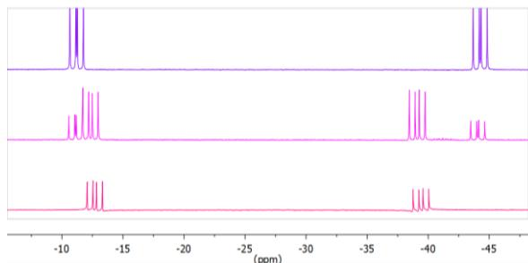
Figure 16.  $^{31}\text{P}\{^1\text{H}\}$  NMR spectra (162 MHz,  $\text{CD}_2\text{Cl}_2$ ) of the evolution of **C2** (bottom) towards **C2-CO** (top).
