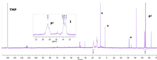
Figure 6.  $^{31}\text{P}\{^1\text{H}\}$  NMR spectrum (162 MHz,  $\text{C}_6\text{D}_6$ ) of **4**.
