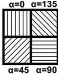
FIG. 1: Representation of the disposition in which are assigned each pixel in the super pixel. [2].
