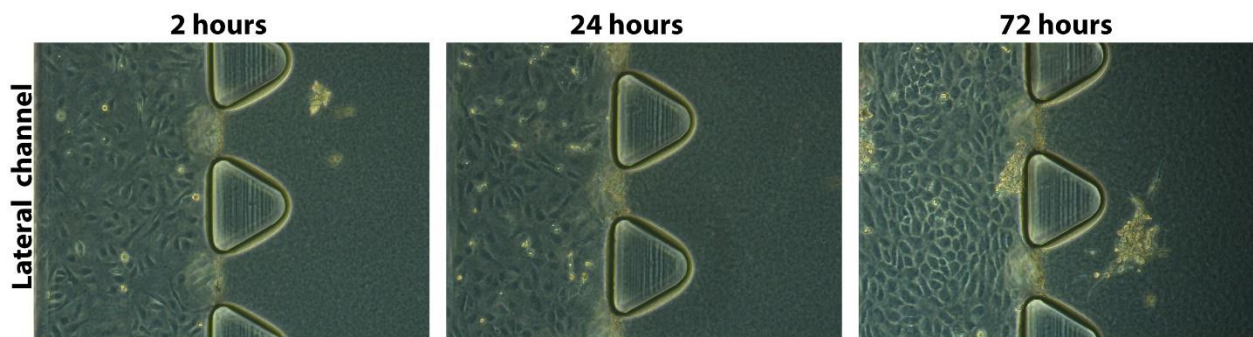
Figure 4.3 HUVECs monolayer formation. Cell growth in the microfluidic chip after 2 hours, 24 hours and 72 hours. Magnified image of the lateral channels (left hand side from the triangular posts) where HUVECs were seeded to form the blood vessel model and part of the gel channel (right hand side from the posts). Distance between triangular posts is 100 \mu\text{m} .
