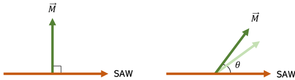
FIG. 5: From left to right. When SAW and magnetization are perpendicular, the magnetization will not have any orientation in which to minimize energy; therefore, it will not move. As the angle changes the lattice motion will have more effect reaching its maximum at 45 degrees.
