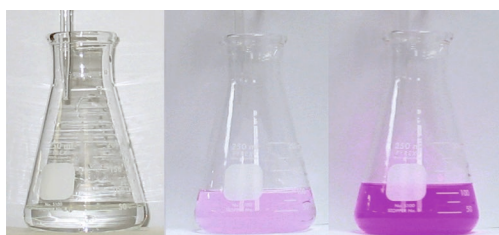
Figure 5. Colour changes of phenolphthalein during acid–base titration of an acid analyte with sodium hydroxide. The middle Erlenmeyer flask shows the optimal colour at the end of the titration.
