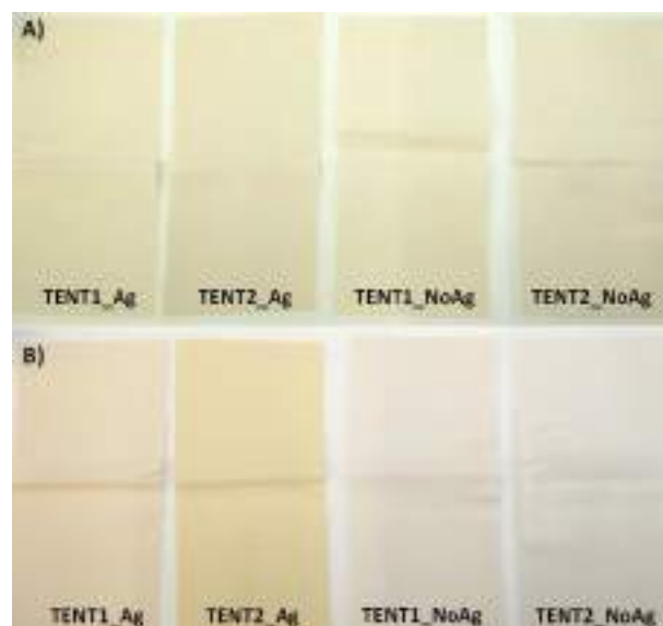
Figure 26 – Visual aspect of the 4 samples. A: Tent exterior side; B: Tent interior side (showing the polyacrylic coatings, see Figure 31 for the meaning of the codes).
