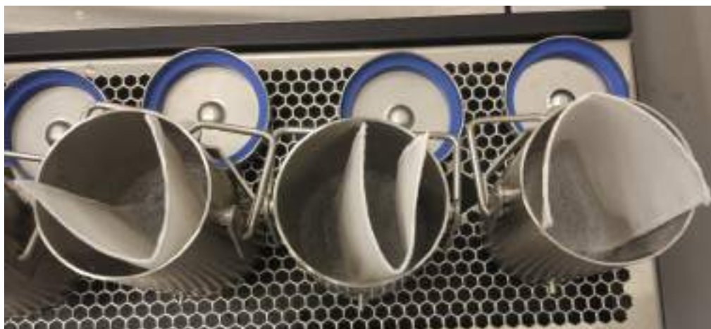
Figure S 2 – Washing vessels containing the textiles, detergent solution and stainless steel balls (not observed because are covered by the foam).
