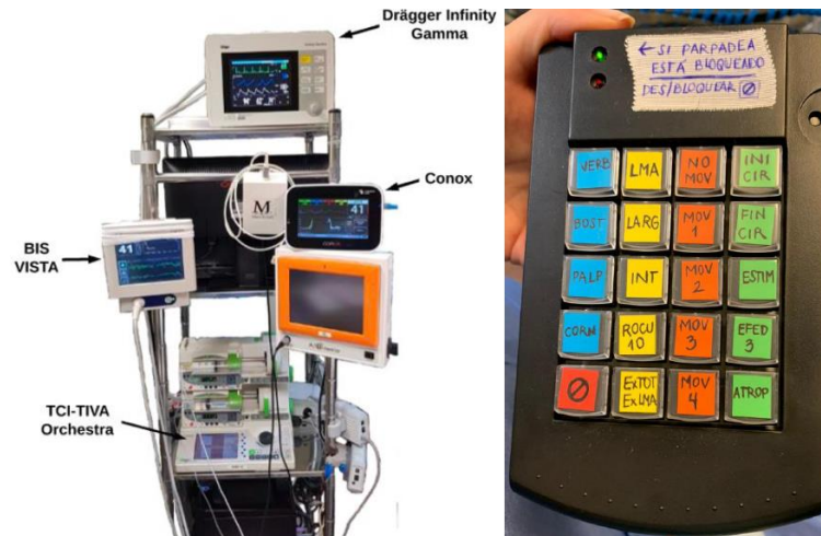
Figure 6. Anesthesia control tower with the monitoring and anesthesia-infusion devices (left) and adapted keyboard for surgery-related events registration (right)
