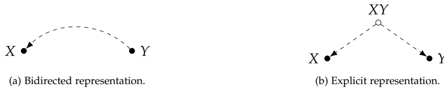
Figure 3.9: X and Y are confounded by an exogenous variable XY , and outgoing edges from X have been deleted (incorrectly in (a)).
