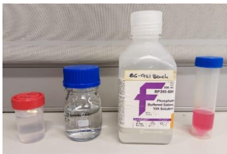
Figure 13: Electrolytes used for EGOFET characterisation. From left to right: Milli-Q, NaCl solution, PBS and DMEM.
