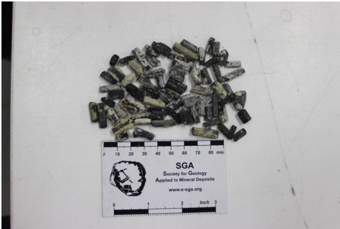
Figure 3. Single euhedral crystals of hornblende. These are selected to help the student to easily identify the three-dimensional shape of the crystals and to discover the shapes of the sections taken in different orientations. The samples are from Carboneras, Almería, Spain.
