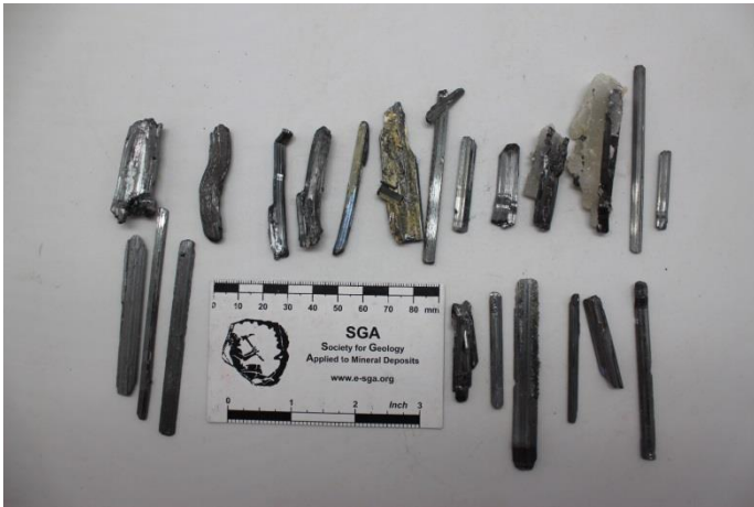
Figure 5. Euhedral crystals of stibnite from China. These are selected to show the ideal prismatic shape of the good-quality stibnite crystals.
