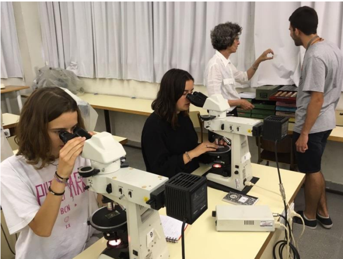
Figure 2. Study of thin sections of mineral assemblages using transmitted and reflected optical microscopy at the laboratories of the University of Barcelona. Some samples are stored in the green plastic boxes at the back of the picture.
