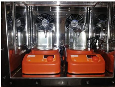
Figure 9: Experimental set-up of the photodegradation of sulfamethoxazole in aqueous suspension of \text{TiO}_2 inside a Solar Simulator
