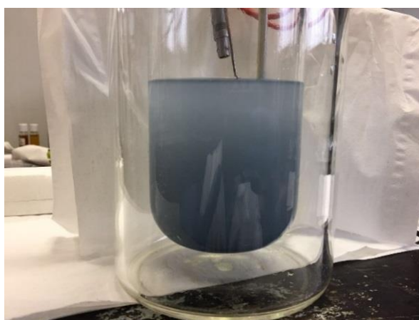
Figure 3.26. The reaction suspension of Ti10-PMO just turning off irradiation after the photocatalytic test of H 2 production from ethanol (aq) 25% v/v at 20 °C.
