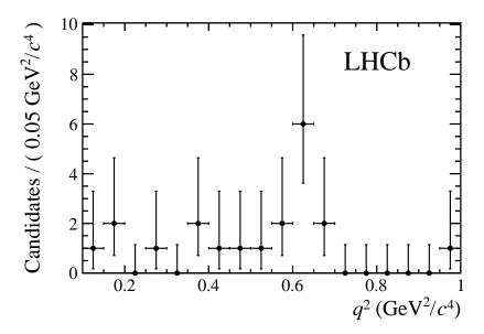
Figure 5: The  $q^2$  spectrum of  $B^+ \to \pi^+ \mu^+ \mu^-$  candidates in the region  $0.1 - 1.0 \,\text{GeV}^2/c^4$  in a  $\pm 50\,$  MeV window around the nominal  $B^+$  mass, showing a peaking structure at  $0.6 \,\text{GeV}^2/c^4$  that is in the region of the  $\rho^0$  and  $\omega$  masses squared.
