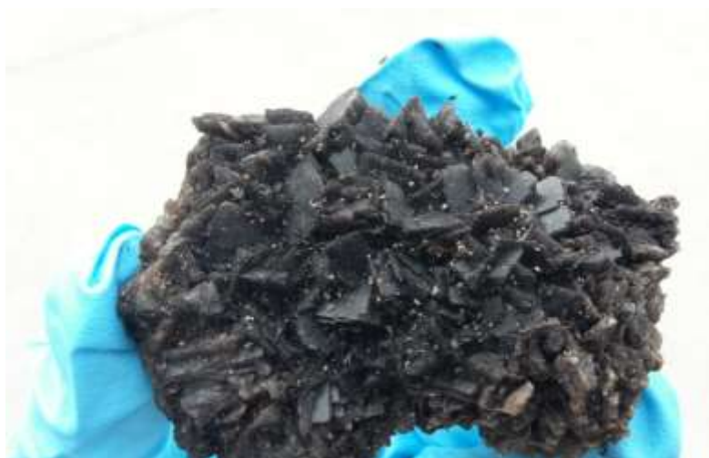
Figure 5.2. Struvite crystal extracted from a pipe in Pineda WWTP.
