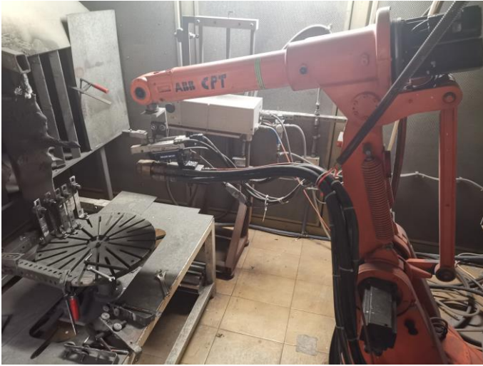
Figure 3. HVOF spraying chamber (CPT Barcelona)
