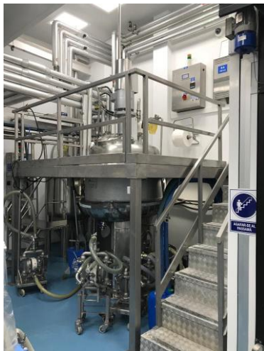
Figure 17: 600L volume reactor made of 316 stainless steel by TEMEC.
