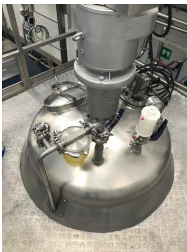
Figure 18: 600L volume reactor made of 316 stainless steel by TEMEC.
