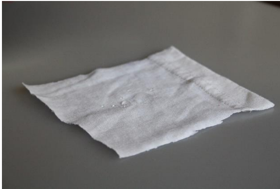
Figure 4. Hydrophilic surface (fabric), contact angle less than 90^\circ
