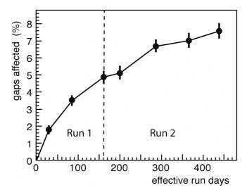
**Figure 5.** Accumulated fractional number of new trips observed in the detector, normalized to the total number of gaps (4944), as a function of the total number of effective run days integrated between 2010 and 2018. The values are evaluated at the end of each year of data taking. Errors are statistical.
