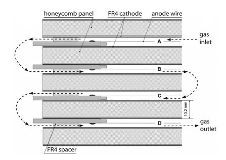
**Figure 2**. Cross section of a MWPC with four gaps indicated by A, B, C and D. The direction of the gas flow is shown by the dashed lines. On the detector, a maximum of 8 MWPCs are connected in series on the same gas line, for a total internal flux from 3 to 16 gas volumes per day, depending on the detector region. It should be noticed that the Muon gas system works in closed loop, recirculating tipically 90% of the gas.
