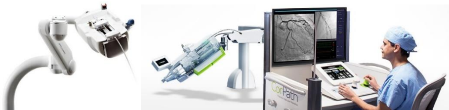
Figure 7. Robotic intravascular systems. On the left, the Sensei System from Hansen Medical. On the right, the CorPath GRX from Corindus.
