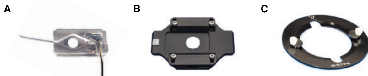
Figure 43. Recording stage set up used for electrophysiological recordings of autaptic neurons. A) RC-25F recording chamber with the perfusion and suction tubes connected to the chamber's inlet and outlet, respectively. These tubes allow external solution to enter and leave the chamber, thus providing a continuous flow. The coverslip was mounted beneath the middle of the chamber (hole) and sealed with vacuum grease. B) P-4 chamber platform to hold the recording chamber. C) SA-OLY/2 stage adapter to assemble the chamber platform onto the objective of the inverted microscope.
