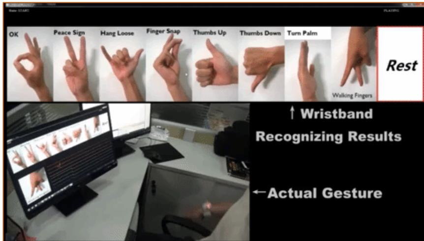
**EMG-IMU Wristband for Hand Gesture Recognition**
