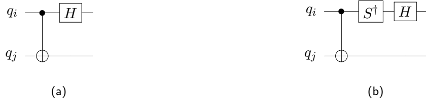
Figure 7: Circuit introduced to make measurements of (a) \{\langle \dots X_i \dots X_j \dots \rangle, \langle \dots Y_i \dots Y_j \dots \rangle\} and (b) \{\langle \dots X_i \dots Y_j \dots \rangle, \langle \dots Y_i \dots X_j \dots \rangle\} .
