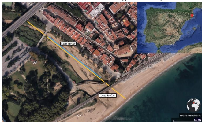
FIG. 3: ERT study location with the measured profiles.
