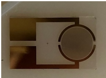
FIG. 2: Image of a fused silica IC, where the pads (left) and interdigitated electrodes (right) can be seen.
