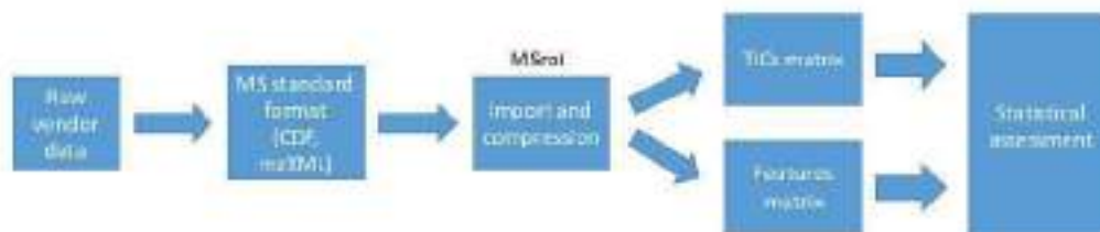
Figure 5. Workflow of the data analysis strategy from the MS raw data acquisition to the statistical assessment.
