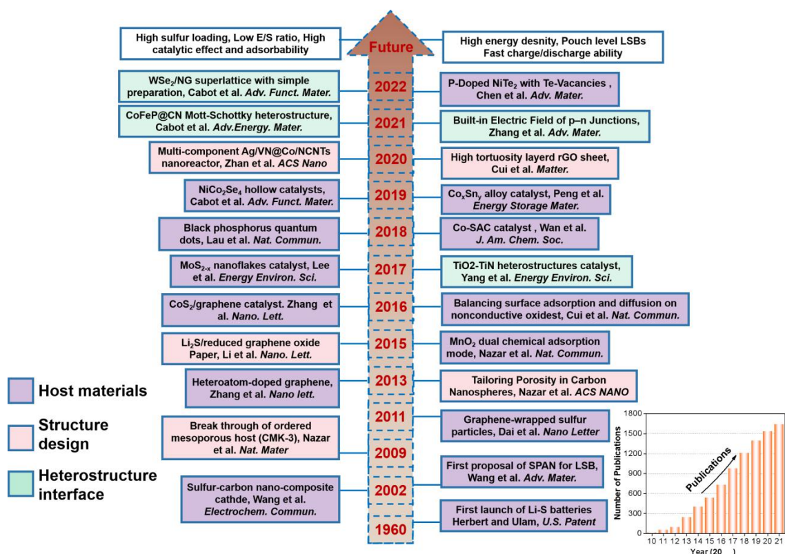
Figure 3. Overview of the development of LSBs from the first proposal to the present. Inset in the lower right corner is the number of publications in recent years with the topic keywords of "Li-S battery" and "lithium-sulfur battery" in the Web of Science database, dated March 1 st , 2022.
