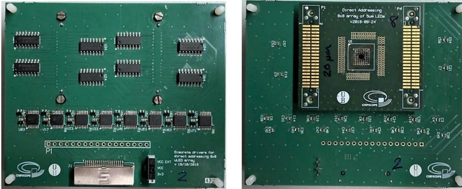
Figure 3.18: Picture of the implemented PCB with the LED driving circuit for the direct addressing nanoLED array. Left, bottom side with the different ICs. At the right, the top side with the nanoLED PCB connected.
