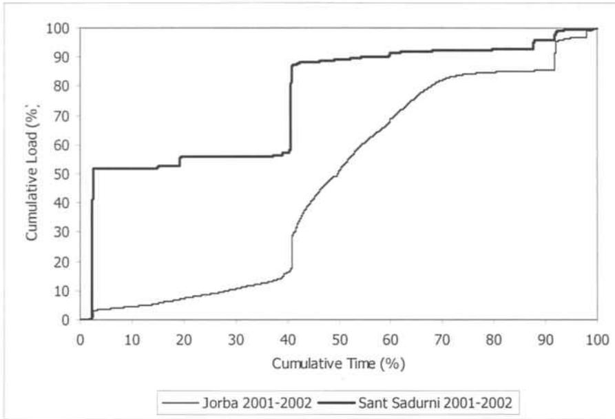
Figure 5-27: Cumulative time against cumulative load during 2002-2003 at both sampling sites
