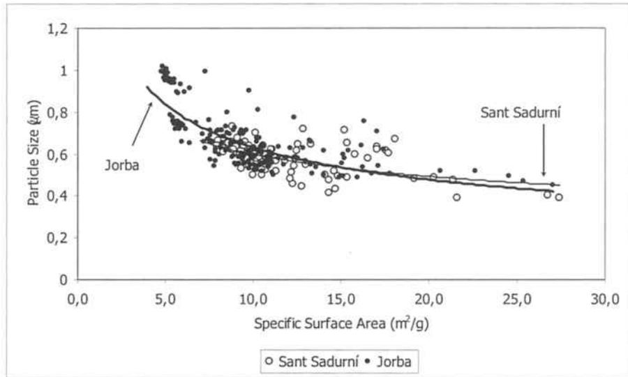
Figure 5-16: Specific surface area and Mean particle size.
