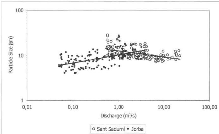
Figure 5-15: Relationship between particle size and discharge at both sampling sites.
