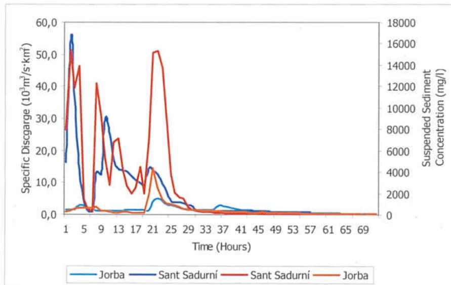
Figure 5-8: Evolution of specific discharge and sediment concentration at both sampling sites during the event.
