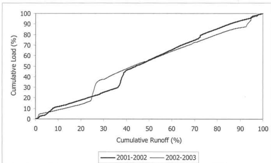
Figure 4.6-8: Cumulative load versus Cumulative Runoff for both water years.
