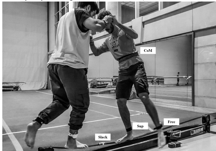
Fig. 1. Slackline task. Accelerometers were placed on the support leg (Sup), the free leg (Free), the center of mass (CoM) and the slackline (Slack).
