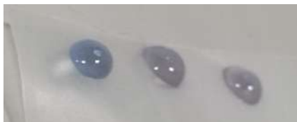
Figure 5: Drops of Coomassie blue (with SDS that denaturalizes the proteins) mixed with the eluate candidate to contain the protein. The eluate was collected when there had flowed: 3, 4 and 5 mL of elution buffer through the column.
