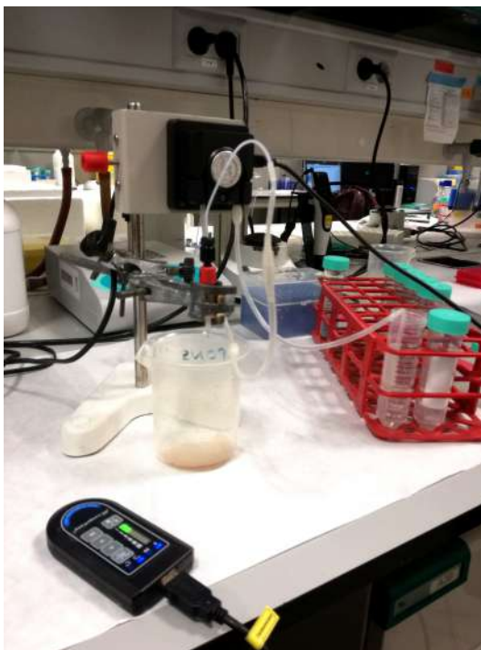
Figure 4: Ni NTA column. The column is connected to a peristaltic pump that allows the fluid to flow.
