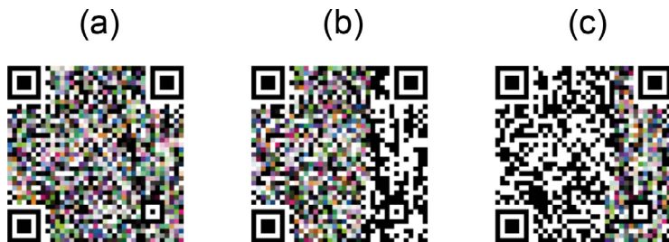
Fig. 5. The same QR Code with data https://color-sensing.com/#000 is populated in different areas with 80% of colors for each area. (a) The whole QR Code is populated (EC&D). (b) Only the error correction area is populated (EC). (c) Only the data area is populated.
