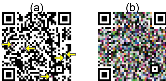
Fig. 2. The same QR Code with data https://color-sensing.com/#000 is populated with different amounts of colors. (a) 1% of the pixels are substituted using a random placement method (yellow arrows show the colored pixels). (b) 100% of the pixels are substituted using a random placement method.
