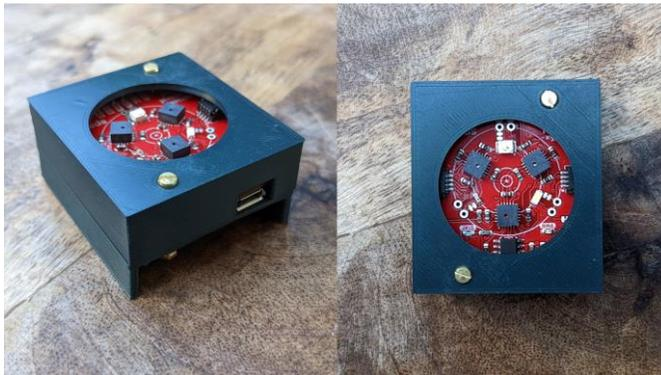
Figure 5-30. Side and top view of the AS7265x module and ATSAM21G18 microcontroller breakout boards.
