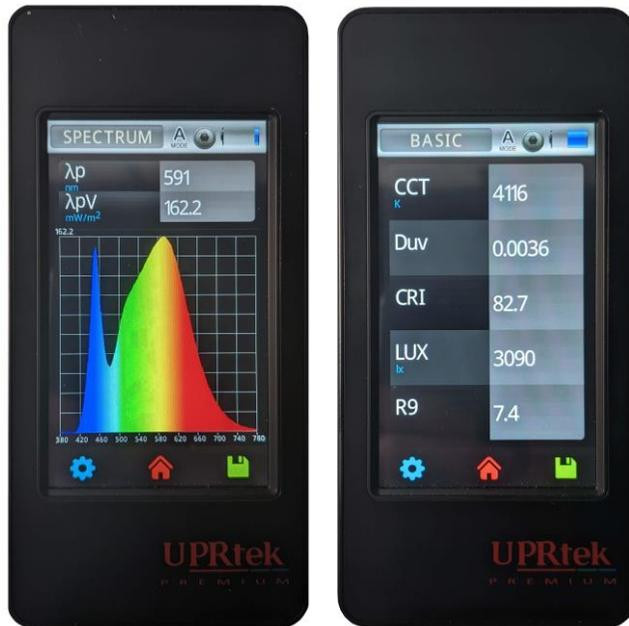
Figure 2-30. UPRtek MK350S premium calibrated portable spectrometer [83].
