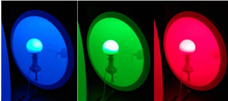
Figure 4-31. Second version of the prototype working within the integrating sphere.
