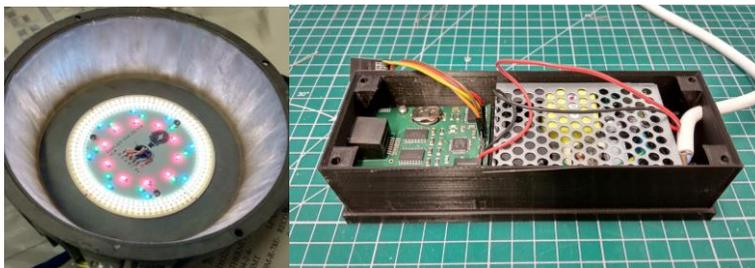
Figure 4-37. Picture of the downlight prototype without the covers.
