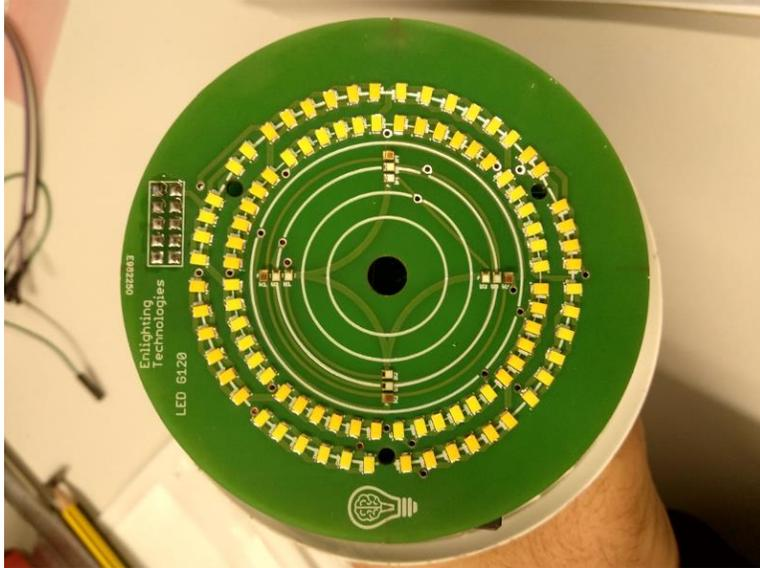
Figure 4-29. Picture of the manufactured LEDs PCB.
