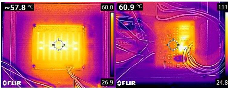
Figure 4-41. Thermal image of the LED module PCB (left) and the control module PCB (right) of the floodlight prototype without the front cover after 20 minutes of operation.
