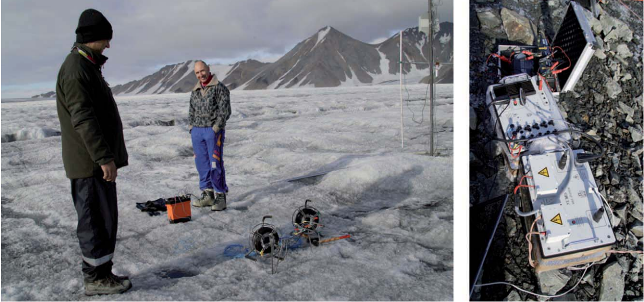
Fig. 5. Ice resistivity measurements (ABEM 4000 device) on stick number 4 at 175 m a.s.l. and image of the used device Numis Lite 005 at the glacier front (30 m a.s.l). Ice is a perfect electrical insulator so the maximum MRS depth is obtained by the loop size and configuration (Photo: O.Hengesch)
