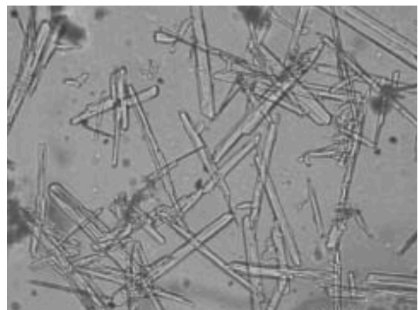
Figura 30. Ciril Pohar. Optical microscope images of the gypsum samples taken from a lime suspension . Recuperat de https://www.researchgate.net/figure/Optical-microscope-images-of-the-gypsum-samples-taken-from-a-lime-suspension-100-g-dm-3_fig8_230163172
