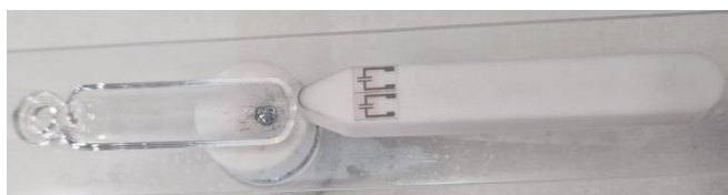
FIG. 2: Image of the experimental layout inside the quartz tube. On the left, the precursor. On the right, the substrates with parallel electrodes.
