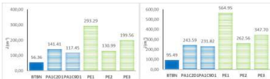
Fig. 28: Comparison between reference A1C1D1 and designed PA1C2D1, PA1C9D1 and PEn structures using either (a) Noodleman's ( J_N ), or (b) Yamaguchi's ( J_Y ) approach to calculate J_{AB} magnetic interactions.
