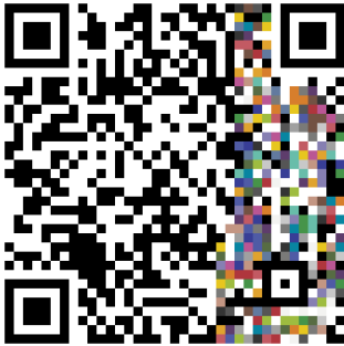
Figure 14: A color QR Code (version 5 with H error correction level) which contains 240 pixels that are coloured. This is implemented with our back-compatible method. These color pixels reproduce the 24 original ColorChecker colors with a redundancy of 10 pixels per color. Only 22% of the digital data pixels are used in this process, almost all the Z_D zone is used to allocate the colors.
