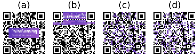
Figure 4: The color information from the ColorSensing logo is distributed using different criteria, each one of these distributions compute different measures of SNR and BER, although the total amount of colors is the same, the way they are distributed affects the signal quality. (a) The original QR Code with the logo. (b) The logo colors are sorted at the top of the QR Code. (c) The logo colors are randomly distributed among the QR Code. (d) The logo colors are distributed by using a threshold criterion among blacks and white colors.
