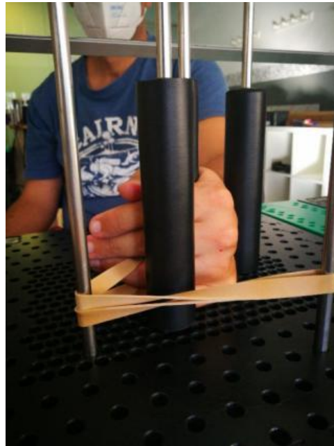
Figure 2. 500 g extension force at 90° applied for fifteen minutes at the head of P2 using a MAPS Therapy Pegboard.
