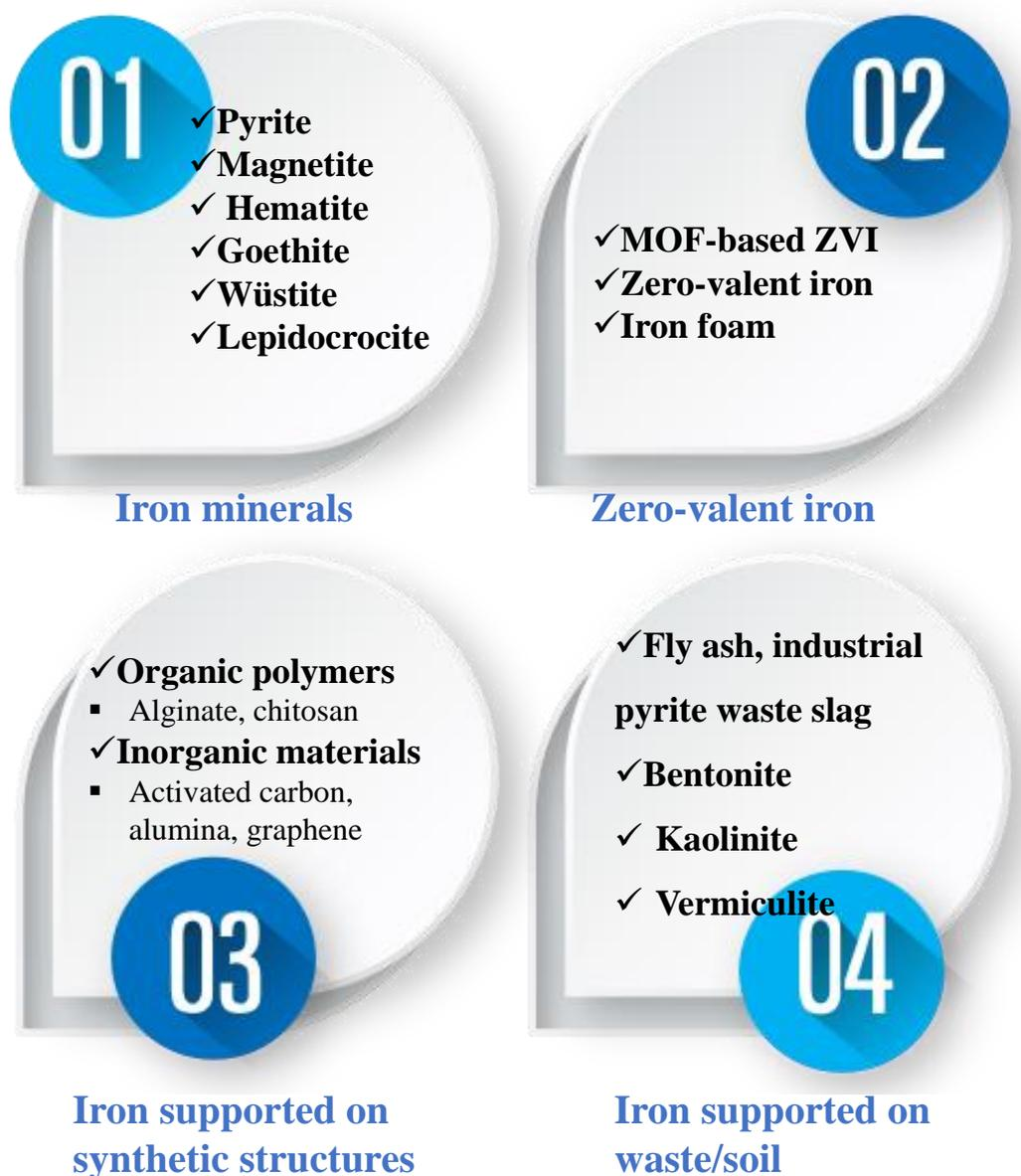
**Fig. 5. The four types of heterogeneous catalysts commonly used in the EF process.**
